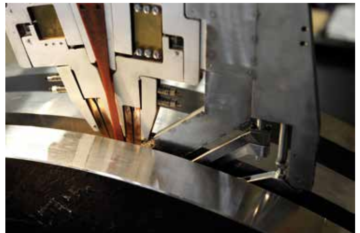
Double-sided joint tracking
