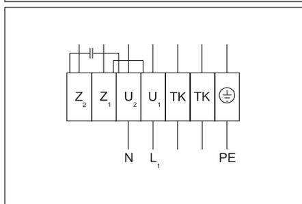
**Wiring diagram No. 2 (1~230V)**
