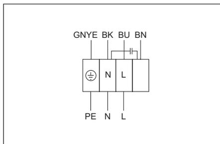
**Wiring diagram No. 1 (1~230V)**
