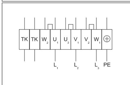
**Wiring diagram No. 3 (Δ - 3~230V)**
