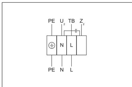
**Wiring diagram No. 4 (1~230V)**
