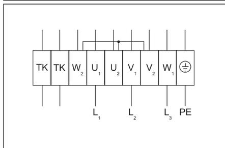
**Wiring diagram No. 3 (Y - 3~400V)**
