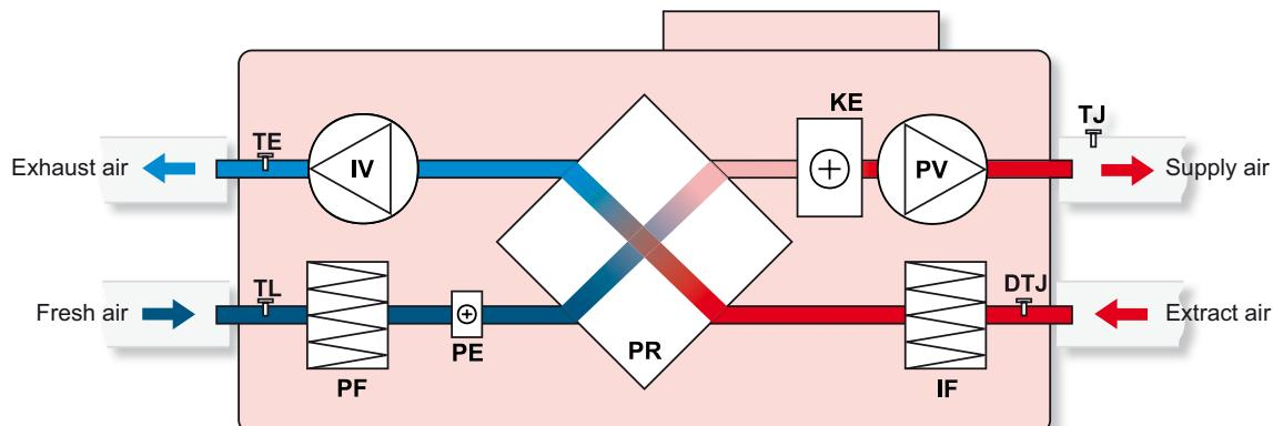
\* - Summer cassette can be applied to RIS 400 PE 3.0; RIS 700 PE 3.0. Used for closing-up of plate heat exchanger during warm period of the year when heat recovery is of no benefit.
