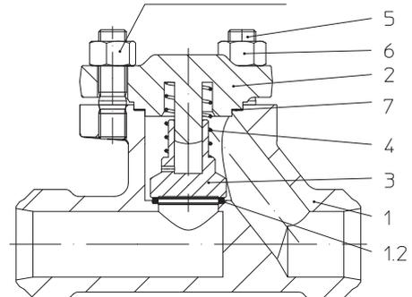
Рис. 6: CHECKO<sup>®</sup>-V - DG SE PN63-160
