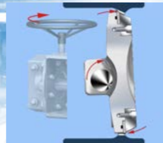
Maximum closing force with minimum effort because the contact angles are optimised with our special geometry optimisation software.
