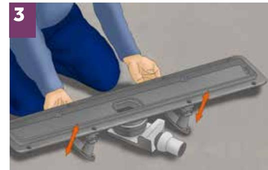
**3** There is a grate holder which is adjusted according to the height with special feet with a screw - pillar.
