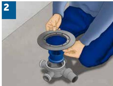
**2** During installation make sure that all rubber seals are lubricated. Inserting of socket into the base (if we are talking about S base, this step does not exist, -S base does not have socket). Setting of a hoop for hydro isolation to the selected base.
