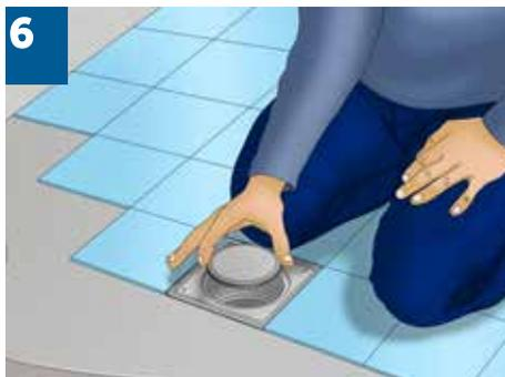
**6** Setting of a temporary safety cover. Setting of tiles on the bathroom floor.
