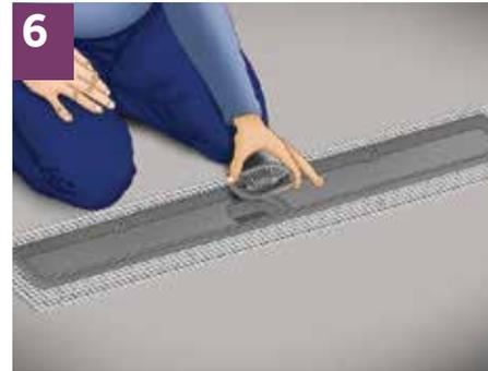
After setting up the hydroinsulation, hair stopper is inserted, and setting up the tiles in the bathroom can start.
