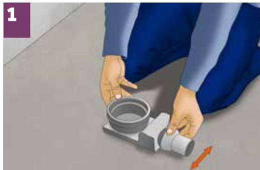
**1** Setting of a base with the ball (output  $\varnothing 50$ ) on the bathroom floor in the proper position. Adjusting the angle of a drain (output) according to the situation in the bathroom.
