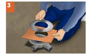
Installation of flange for hydro isolation. Between it and hoop, hydro isolation is inserted.
