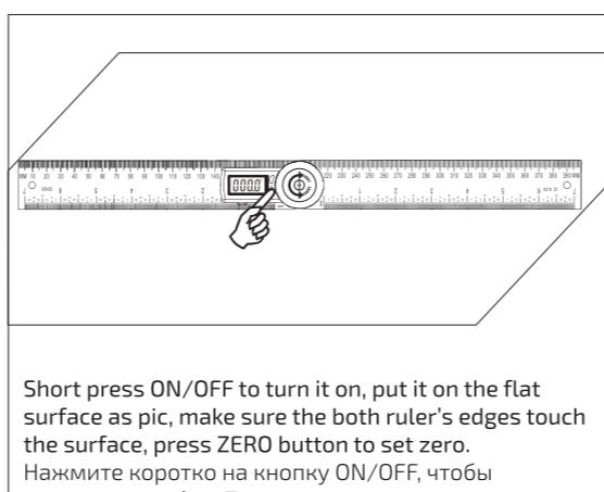
Short press ON/OFF to turn it on, put it on the flat surface as pic, make sure the both ruler's edges touch the surface, press ZERO button to set zero.
