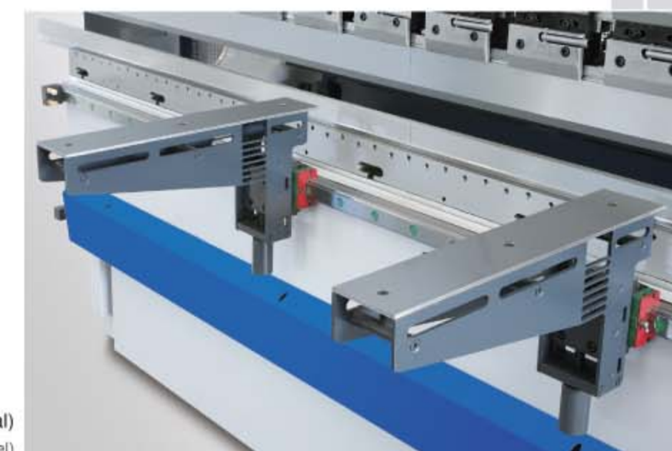
Multiple sheet support locations (standard) Supports avant a multiples emplacements (standard)
