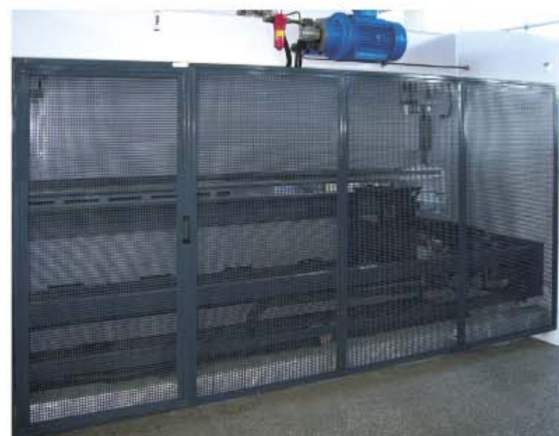
Rear fence-type guarding (standard) Garde arrière de type grillage (standard)
