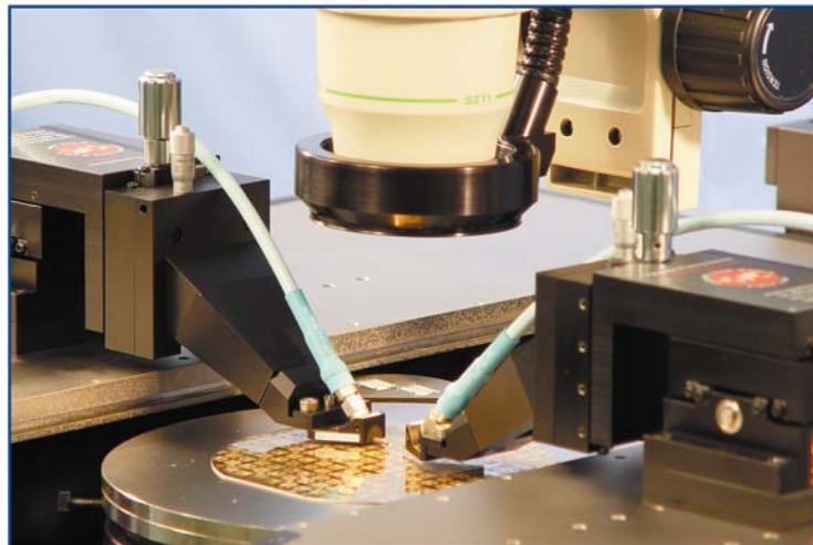
The WL-210 calibration chuck offers 3 substrate sites which support either landscape or portrait format calibration substrates.
