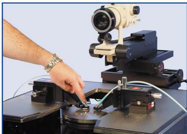
The tilt-back microscope provides unobstructed fixturing access.
