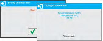
Upon confirmation of serial number START message is displayed. Press key to confirm. The drying process starts and continues until specified temperature is reached. Time and sensor temperature information is displayed.
