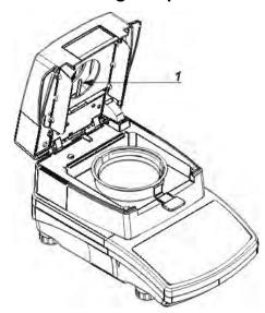
To ensure correct temperature measurement make sure that the temperature sensor is clean (1).
