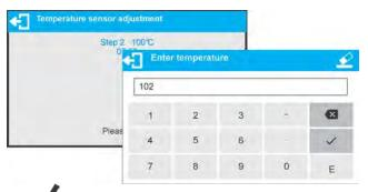
Press \ key to confirm, the third step of adjustment starts. The moisture analyzer halogen lamp starts to operate and the drying chamber is heated as long as necessary to provide specified temperature, which is next maintained for 8 minutes. After 8 minutes a numeric keyboard is displayed. Enter the moisture analyzer temperature that is displayed on the control thermometer.
