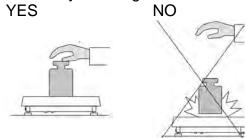
Place weighed loads centrally on the weighing pan:
