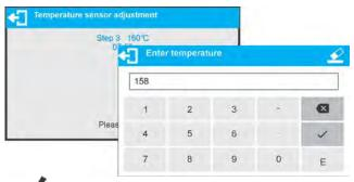
Press **V** key to confirm. Temperature adjustment process is completed and moisture analyzer displays <Adjustment> window.
