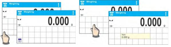
• A new widget can only take such area that holds no other widgets yet. The software automatically detects which widgets can be applied for a particular area, this is conditioned by widget dimensions.
