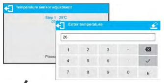
Press key to confirm, the second step of adjustment starts. The moisture analyzer halogen lamp starts to operate and the drying chamber is heated as long as necessary to provide specified temperature, which is next maintained for 8 minutes. After 8 minutes a numeric keyboard is displayed. Enter the moisture analyzer temperature that is displayed on the control thermometer.
