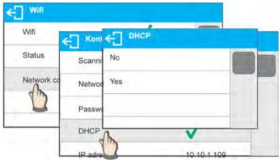
With DHCP set to NO value, enter manually: <IP>, <MASK>, <DEFAULT GATE> parameters.
