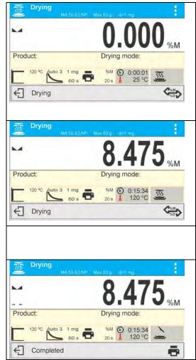
Information on the drying process is displayed, moisture analyzer proceeds to carrying it out accordingly to set parameters. Required mass measurements and calculations of tested sample moisture content are performed, wherein the calculations are a result of mass change. On process start, printout header is sent to a selected interface (accordingly to set printout options – parameter group DRYING PROCESS REPORT/HEADER).
