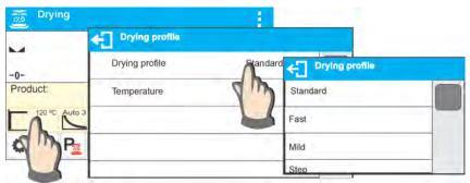
Enter drying parameters settings and select mode type. Upon selection fields enabling setting profile parameters are displayed. Parameters depend on selected mode.
