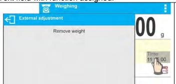
Press to develop an internal adjustment operation (internal adjustment function is assigned to the text field).
