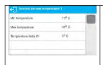
Min temperature – min balance temperature, for lower temperature values the thermometer pictogram is red Max temperature – max balance temperature, for higher temperature values the thermometer pictogram is red Temperature  $\Delta t/h$  – maximum balance temperature change rate, for higher change rate values the balance displays blinking red thermometer pictogram
