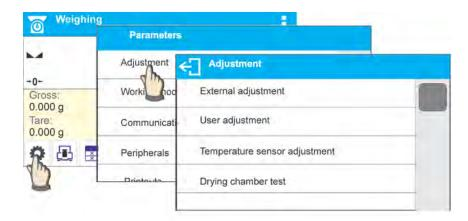
In order to enter balance menu, press <a>PARAMETERS></a> button. Clicking any button comprised within information section, or clicking any button with particular parameter name, results with change of colour. This is for signalling purposes. If a given area has any function or action assigned, then it is performed automatically upon clicking (e.g. adjustment procedure), respectively a particular window with parameters or list of appropriate settings is displayed.
