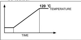
• **STEP drying profile** - For step profile, set heating time in temperature number one, first step temperature, heating time in temperature number two, second step temperature and temperature in which a sample is to be tested.
