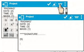
If you want to carry out HEADER or GLP or FOOTER printout using EPSON printer (equipped with autocutter blade) and crop the paper beneath the respective printout, then you have to select an option of non-standard printout comprising {151} variable, and set this option in header, GLP printout or footer settings, respectively (means for entering control codes are described in section 21 of this user manual).
