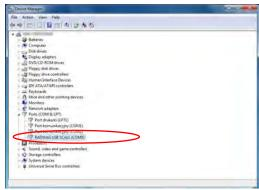
For this very case it is STMicroelectronics Virtual COM Port (COM8). Set balance parameters: select USB value for parameter COMPUTER/PORT. Run software for measurement readout.
