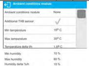
Ambient conditions module – parameter specifying module's working mode. Available options: None – readout of ambient condition module indications turned off; Record - readout and record of indications into database turned on, Record and alert – readout and record of indications into database turned on, option of display of warnings informing on ambient conditions change turned on, the warnings are displayed in accordance with the following tolerance values settings.
