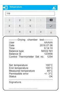
The temperature is maintained for 8 minutes (like for temperature adjustment procedure). After 8 minutes you shall see a window for entering temperature read from the installed adjustment set. Press v to confirm.
