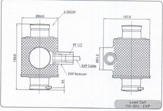
Truck and Tank Weighing Load Cell
