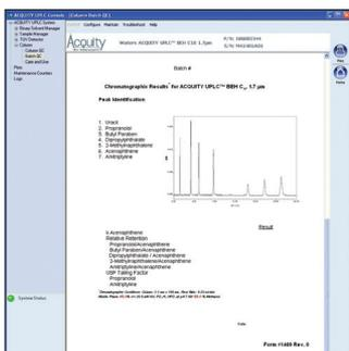
The eCord chip provides the user with QC test conditions and results on the column run by the manufacturer. The information includes mobile phases, running conditions, and analytes used to test the columns. In addition the QC results and acceptance is placed onto the column.
