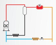
pRack Hecu can manage a solenoid valve as an alternative to the EEV valve for liquid injection.
