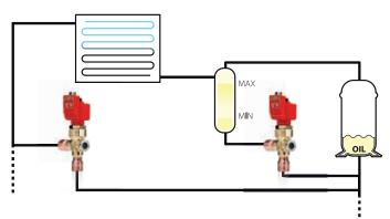
By installing an advanced oil separator with double level sensor, the E2V valve control algorithm makes sure the exact quantity of oil required by the system is injected.
