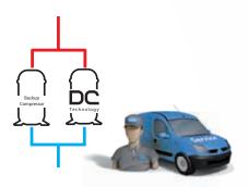
High service level with backup compressor activated only in the event of alarms or malfunctions on the main compressor. The system continues operating and service response times are less critical.
