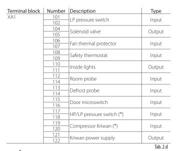
(\*) Warning: if input 117-118 and/or 119-120 are not connected, the control will show an "IA" alarm.
