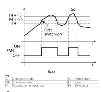
Note: if no condenser probe is selected, the condenser fan output is deactivated.
