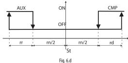
Reverse operation (r3 =2), in the case of 1 compressor output (CMP) r3=2
