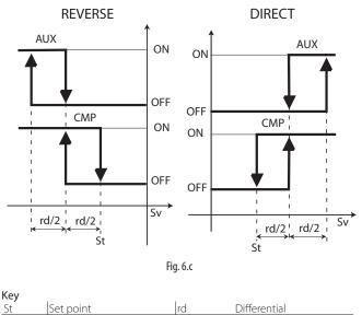
The neutral zone is activated on the controller only if the reverse output is activated with neutral zone control, H1 = 11.
