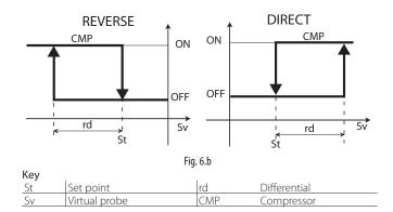
If the second compressor output is activated (H1 = 12) on the AUX output, the compressor output is activated at  $St\pm rd/2$  and the AUX output at  $St\pm rd$ , as illustrated in the following figure.
