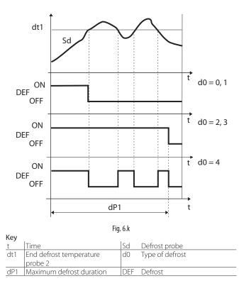
Heater defrost by time with temperature control (d0=4) is used to activate the defrost output only if the evaporator temperature (Sd) is less than value of the parameter dt1, and ends after the time defined by dP1. This function is useful for energy saving.
