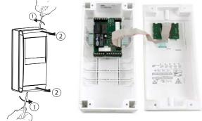
1. Remove the faceplates (1 and 2) and unscrew the screws to open the control
