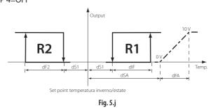
Cooling/heating control for air-conditioner/boiler systems. The analogue output is associated with cooling or heating control, as set ny DIP 4 when LE=2.
