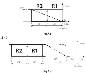
Two-stage temperature control only in heating mode. In cooling mode the situation is diametrically opposite with reference to the set point.
