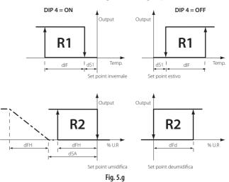
Temperature (top) and humidty control mode (bottom) when LE=2.
