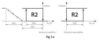
Temperature (top) and humidty control mode (bottom) when LE=2.
