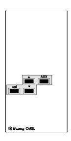
The green zone of the remote control unit reproduces exactly the keypad of the IR instruments and allows you to perform the same operations, as you would perform if you were using the keypad. Here are the main functions of the buttons:
