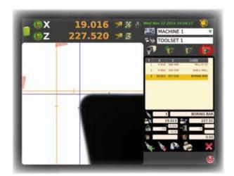
Td SIX is a new additional software function developed by Elbo Controlli, used to acquire tool's measurements, to input them into the tooling tables and create a file including tools offstes.
