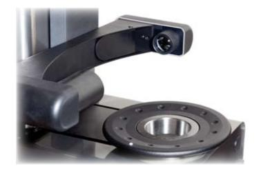
Camera system for measuring and inspection procedures. C-MOS sensor, punctiform and toroidal red light double illuminator. Telecentric optic system with low F/Number.
