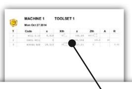
It's possible to generate and / or print a report with the theoretical values, tolerances and measurements of the selected tool table.
