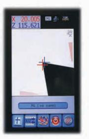
Automatic cutting edge measure. After having found the central position by means of focus bars, on the axes counters the measurement is shown without additional operations.
