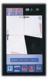
Tool profile collimation on fix reticule with X and Z axes analog comparators: axes control bars for the exact central position of the measure.
