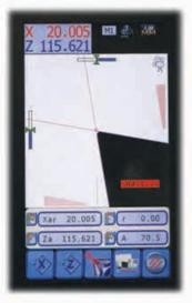
Autotargeting measurement: the viewed profile of the geometrical entities are automatically detected. The values of radii, angles, X and Z axes can be stored and/or printed on the label.
