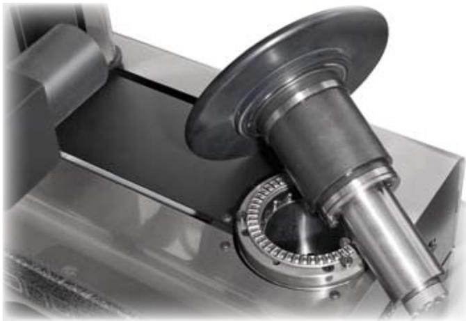
*Interchangeable revolving spindle with mechanical rotation brake.
