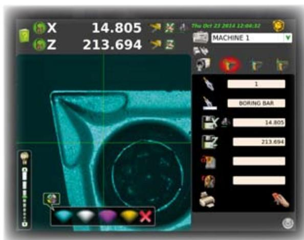
*Inspection function for accurate control of the tool status. Possibility to increase or decrease the brightness for a better visibility.*
