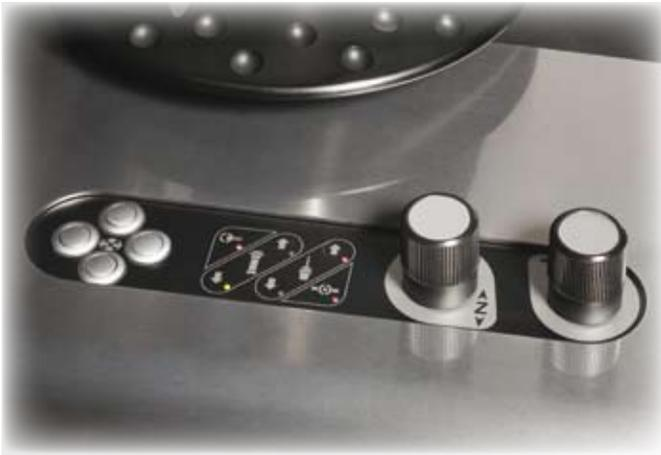
*Stepper motors servo control the axes movements and provide two operation modes: rapid (2.5 m/min) and fine micrometric mode (positioning accuracy 0.8  $\mu\text{m}$ ).*
