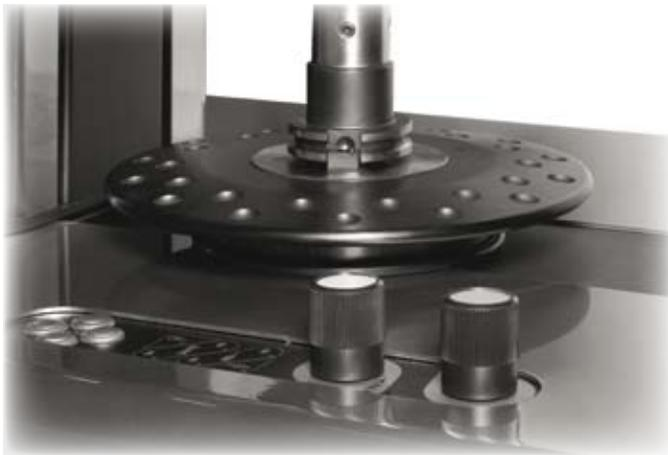
*Micrometric movements (electronic handwheels) are used to collimate the tool profile and to acquire the measurement. The automatic clearance recovery system is patented.*
