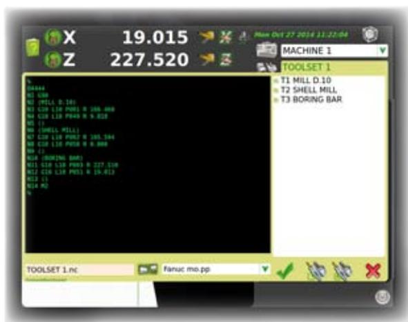
*The datas are elaborated and post-processed by the software. There are more than 50 post-processor format for the most common numerical controls available on machine tool market.*
