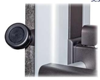
The ergonomic design and location of manual axis movements and controls allow for fatigue-free working. Simultaneous unlocking of both axes is activated by a single button. This operation for locking/unlocking of the axes is pneumatic. Bronze internal sectors act on the screw itself for both axes and have been designed to obtain high-precison fine adjustments.
