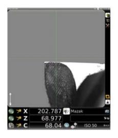
New electronics: a powerful PC running Ubuntu 14,04 LTS for the integrated management and control of the all the functions of measurement/tool inspection, machine origins and tool tables. Ease of use thanks to the integrated touch-screen.
