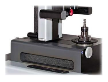
The base and the column, made of ground granite, are increased substantially in size over the previous generation model to guarantee and maintain maximum accuracy. The low coefficient of thermal expansion from this natural material allows the location of the machine directly in the workshop with no issue or concern in respect of accuracy and performance.
