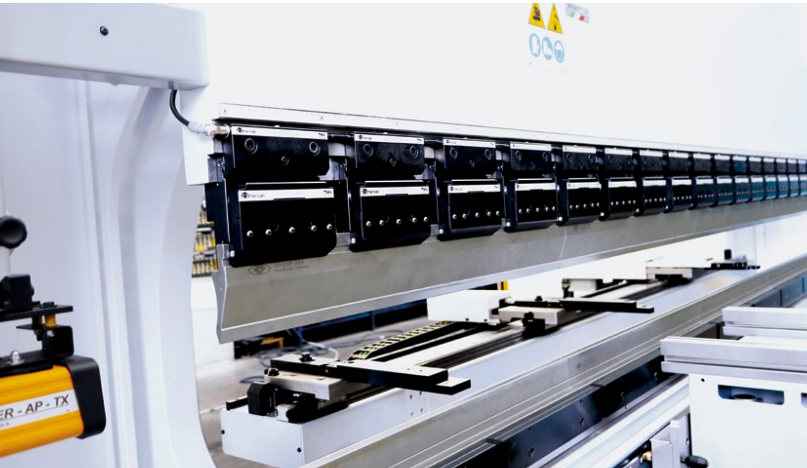
Pneumatic clamping on top and bottom tool.
