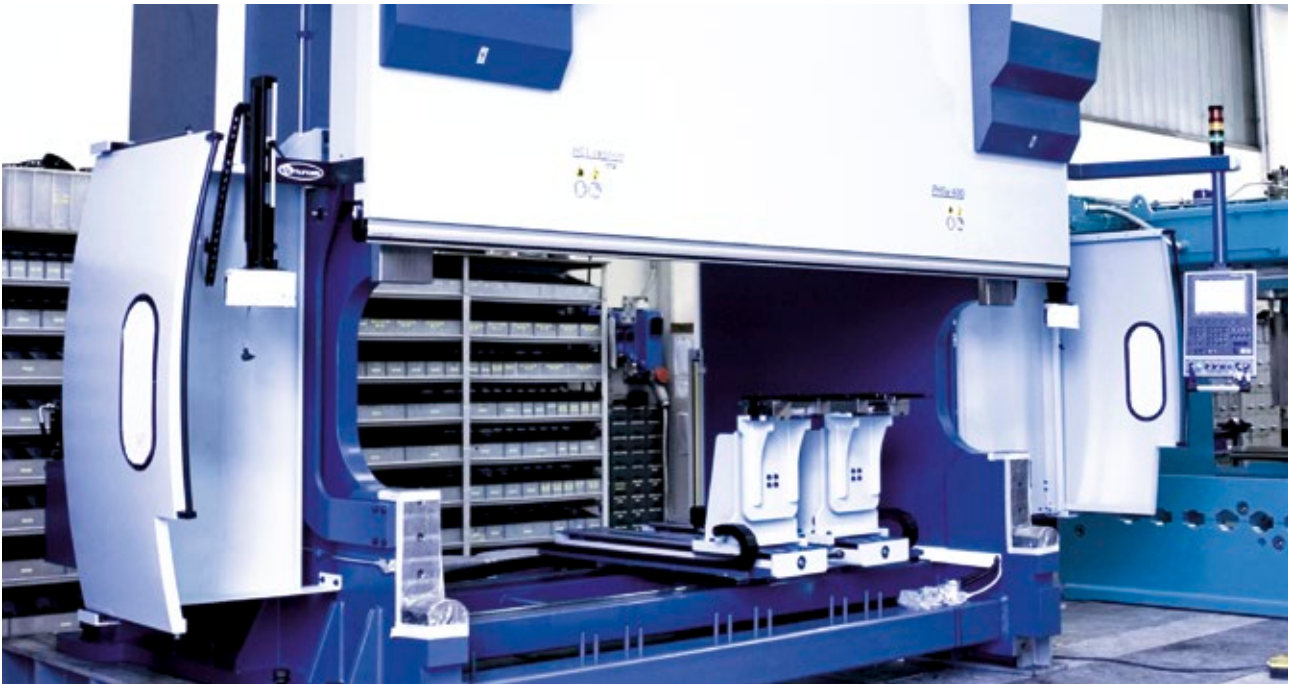
Back gauge system with 6 axes X1-X2-Z1-Z2-R1-R2
