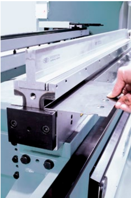
Bending-flattening tool controlled by the CNC.
