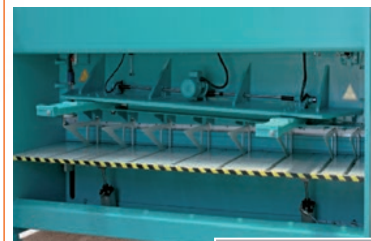
Pneumatic double rear support up to 6 mm with rolls in Teflon to avoid scratching of material with plastic protection.
