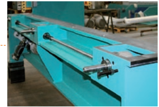
Motorized adjustment of blade clearance.
