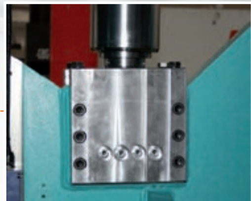
Connection of the shearing beam and the cylinders with adjustment in oil bath.
