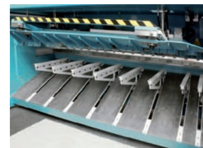
Rear support with teflon protection. The sliding table will be closed completely by the support arms to prevent small parts to get squeezed.
