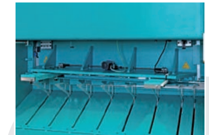
Pneumatic sheet support up to 6 mm.
