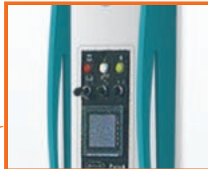
Control panel movable over the machine length.
