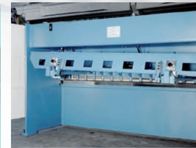
Manual hinged back gauge for cutting large parts extending beyond the travel range of a standard back gauge.
