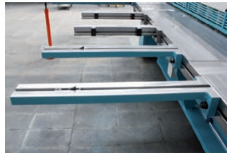
Front supports with disappearing stops.
