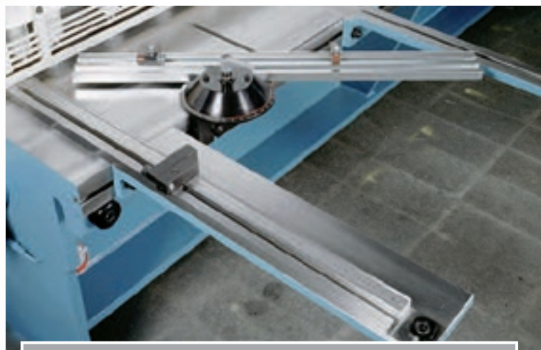
Squaring arm with stop and cutting angle device.
