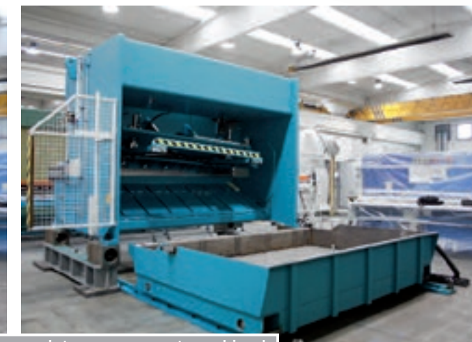
Guillotine shear with heavy duty rear support combined with hydraulic hinged back gauge and motorized evacuation system
