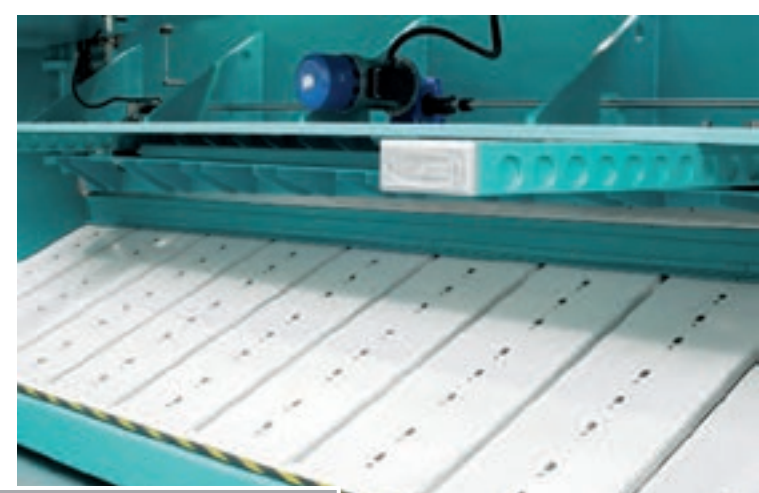
Pneumatic double rear support up to 6 mm with rolls in Teflon to avoid scratching of material with plastic protection.
