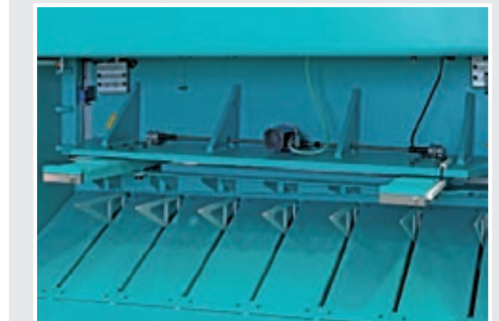
Hydraulic double rear support for heavy material.
