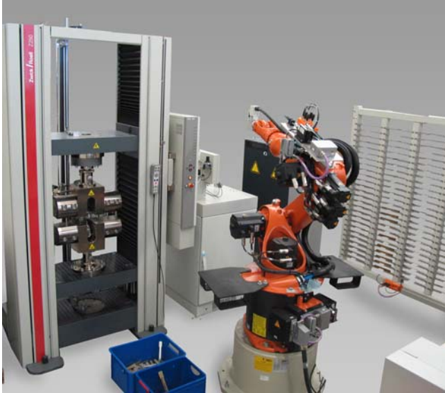
Robotic testing system 'roboTest R' for testing of metals
