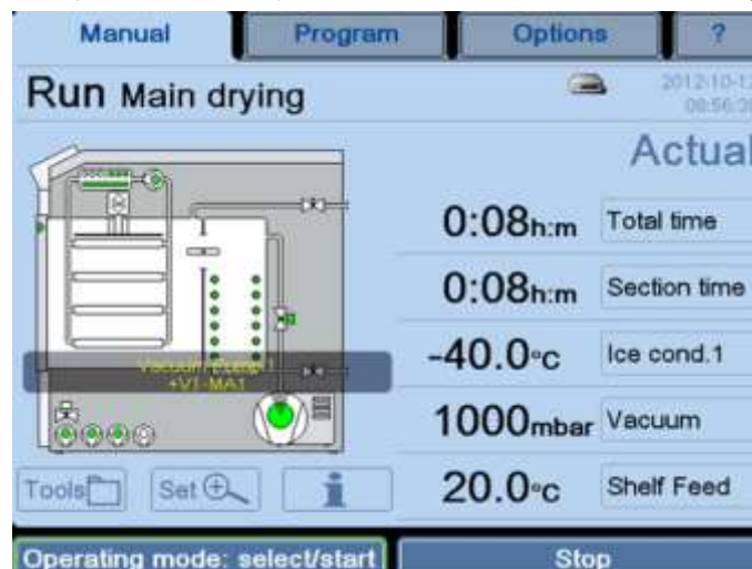
Fig. 30: Schematic system diagram with the name and reference designator of the component
