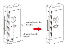
Note 1: Align the template along the vertical center line of the latch(D) at the desired handle height, and tape it to the door.
