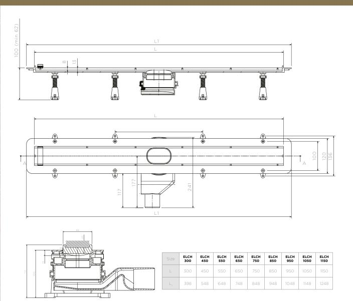
Thanks to new design of holder of grid, all condensed and leaked water under the tile finds it way back to the drain. In complete with self - adhesive butyl tape comes with product and makes Anti Leaking System.
