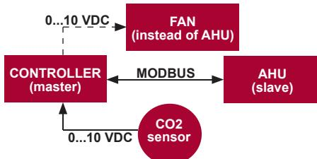
This controller allows controlling level of carbon dioxide (CO<sub>2</sub>) in a room. Connect 0..10VDC CO<sub>2</sub> sensor directly to the controller and configure the controller. In service mode, in item F.14 set 2, and F.15 and F.16 should be set based on the sensor specification.
