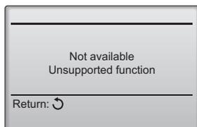
The message at left will appear if the user selects a function not supported by the corresponding Lossnay unit model.
