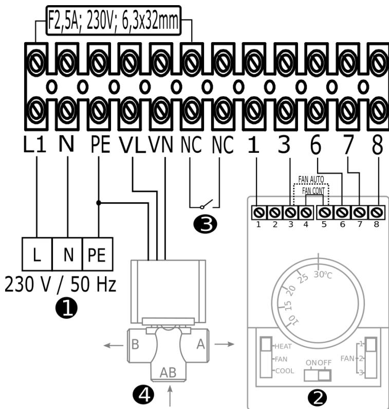
① Power supply 230V/50Hz (OMY 3x1,0 mm<sup>2</sup>) | zasilanie 230V/50Hz (OMY 3x1,0 mm<sup>2</sup>) | stroomvoorziening: 230 V/50 Hz (3-aderig, min 3x1,0 mm<sup>2</sup>) | питание 230В/50Гц (ОМЫ 3x1,0мм<sup>2</sup>)
