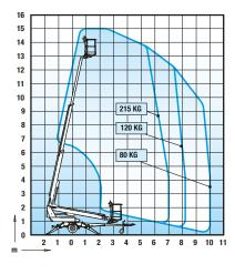
Max. working height 15.00 m Max. platform height 13.00 m Max. outreach 10.00 m Support width 3.8 /4.2 m Lifting capacity 215 kg Basket size 0.70 x 1.30 m Boom rotation cont. 90° Basket rotation Boom control proport. Transport length 6.43 m Transport width 1.78 m Transport height 2.14 m 1670 kg Weight Driving system std AC-socket std Electro motor std Petrol power pack opt. Gradeability 25%
