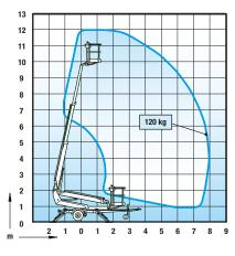
Max. working height 12.00 m Max. platform height 10.00 m Max. outreach 7.90 m Support width 3.15/3.55 m Lifting capacity 120 kg 0.75 x 0.80 m Basket size Boom rotation cont. Boom control 2-speed Transport length 5.52 m Transport width 1.72 m Transport height 1.96 m Weight 1285 kg Driving system std AC-socket in the basket x 2 std Electro motor std Petrol power pack Gradeability 25%
