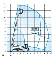
Max. working height 13.50 m Max. platform height 11.50 m Max. outreach 9.10 m Support width 3.8 /4.2 m Lifting capacity 215 kg 0.70 x 1.30 m Basket size Boom rotation cont. Basket rotation Boom control proport. Transport length 5.94 m Transport width 1.78 m Transport height 2.14 m Weight 1635 kg Driving system std AC-socket std Electro motor std Petrol power pack opt. Gradeability 25%
