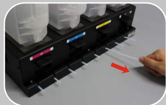
10. Pull out a each ink tubing on the bottom.
