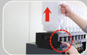
15. After each cartridge is filled with ink, remove each tank by pushing down a lever.
