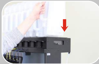
14. Push in each tank to the stand corresponding each color
