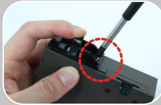
2. Mount a cartridge connector on each cartridge.
