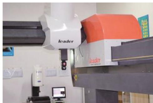
Adopts coordinate measuring machine to guarantee spare parts precision
