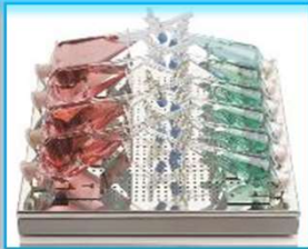
Clamps for Separating funnels
