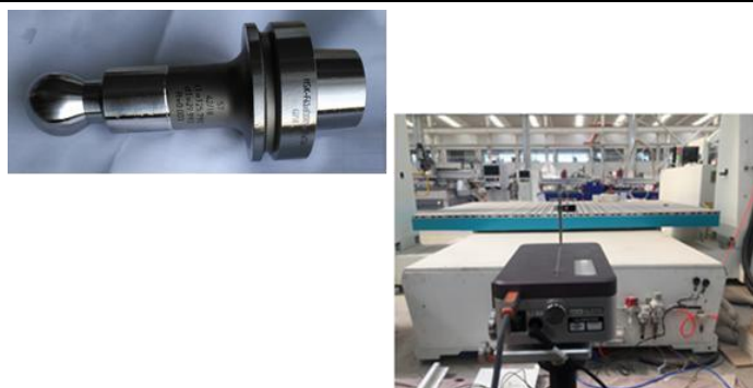
Test bar for RTCP testing from Germany before shipment UK Laser interferometer accuracy testing before shipment
