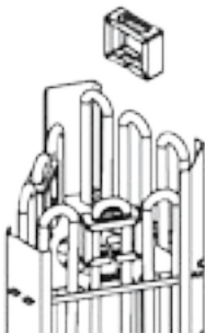
Vastuspidikkeet Heating Element Separator
