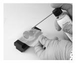
Apply a couple drops of lens cleaning fluid to the lens paper (far side of the lens).
