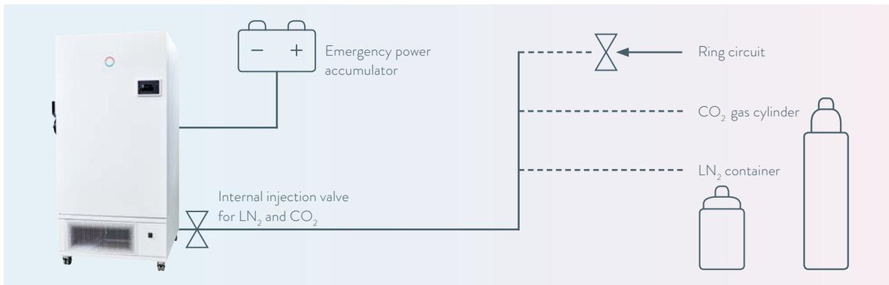
CO<sub>2</sub> or LN<sub>2</sub> connection diagram: Installation of a freezer in a central ring circuit or decentralized installation directly on an emergency gas supply
