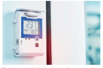
The data logger can be fixed to Versafreeze deep-freezers magnetically and configured or read via a USB interface  $\frac{1}{2} \sum_{i=1}^{n} \frac{1}{2} \sum$
