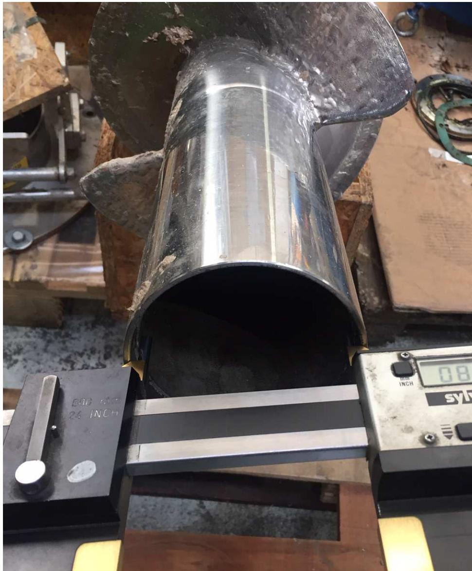
Figure 10: Measure inner diameter
