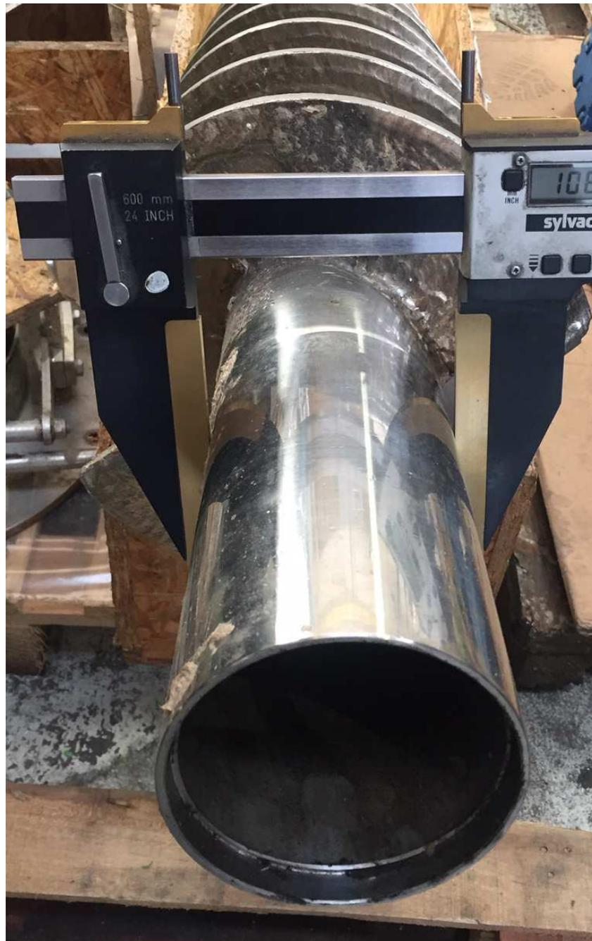
Figure 11: Measure the smallest outer diameter
