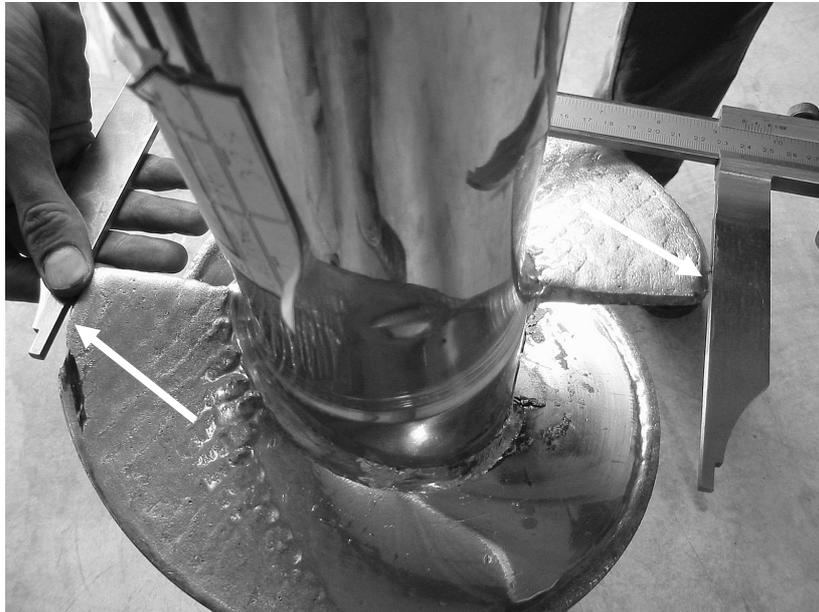
Figure 9: Auger with wear in the press zone and diameter lower than 245 mm
