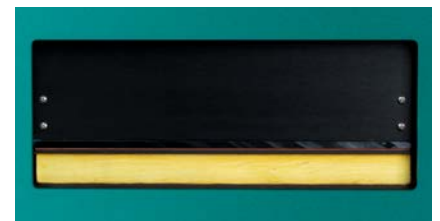
Various plate openings of the HFM 446 Lambda are possible when changing the specimen
