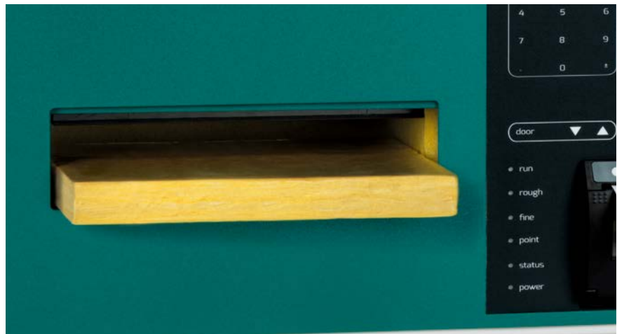
Inserting the reference material; various reference materials can be used
