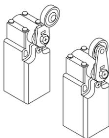
It's possible to fasten the lever on switches on straight or reverse side, maintaining the positive coupling. In this way it is possible to obtain two different work plans of the lever.
