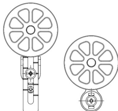
Different actuators with rubber rollers are available. The customer can choose the most suitable product depending on his needs. For example the lift speed in order to reduce the noise inside the cabin.
