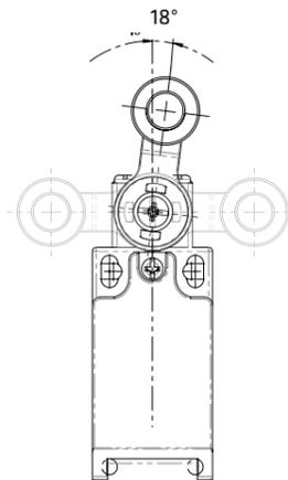
In switches with revolving lever it is possible to adjust the lever with 18° steps for the whole 360° range. The positive movement transmission is always guaranteed thanks to the particular geometrical coupling between the lever and the revolving shaft.
