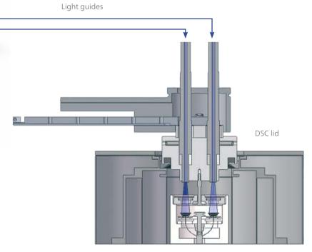
DSC sensor with sample and reference pan
