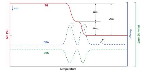
Measured signals in a TGA-DTA
