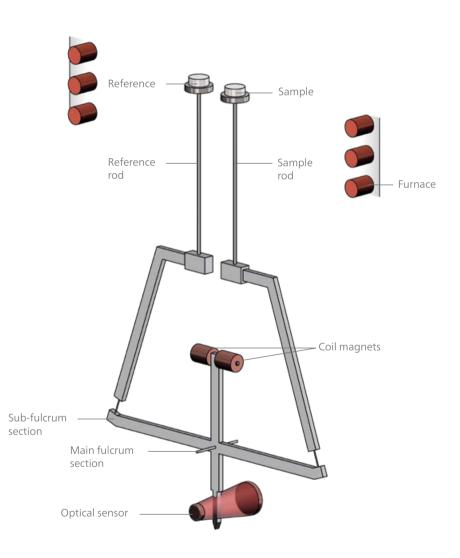
Schematic design of the top-loading differential balance of the STA 2500 Regulus
