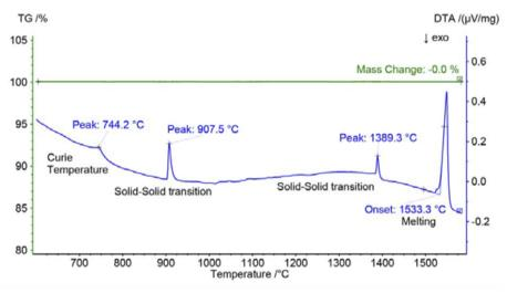
STA measurement of pure iron at a heating rate of 20 K/min. The phase transitions (blue curve) occurred without mass loss which indicates a high purity of iron and no oxidation due to the vacuum-tight design of the instrument.
