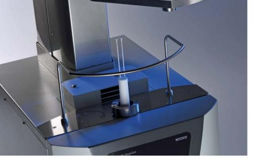
Simultaneous thermal analysis refers to the simultaneous application of two or more thermoanalytical methods to the same sample in one instrument. This term, however, is in most cases used for simultaneous measurement of the mass changes and caloric effects on a sample under thermal treatment.
