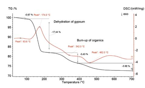
STA measurement on an aged gypsum board (8.32 mg) in air atmosphere (80 ml/min) at a heating rate of 40 K/min in open alumina crucibles. Here, the DTA signal is converted in mW/mg (DSC).
