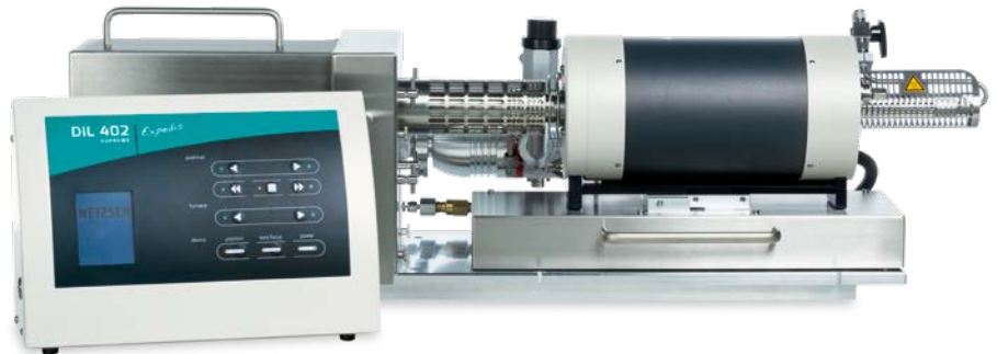
DIL 402 Expedis ® Supreme Glovebox Version with remote control unit (option) for use outside the glovebox
