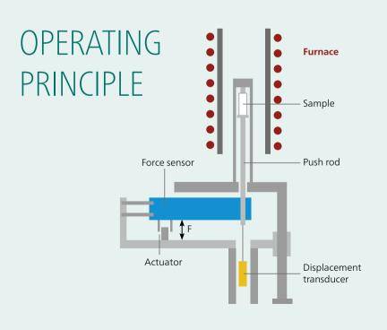
Irrespective of the type of deformation selected (expansion, compression, penetration, tension or bending), every length change in the sample is communicated to a highly sensitive inductive displacement transducer (LVDT) via a pushrod and transformed into a digital signal.
