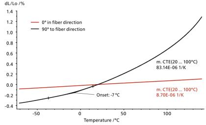
Composite material, measured in two directions; sample length 25 mm, heating rate 5 K/min from -70°C to 140°C,  $\rm N_2$  atmosphere, sample holder made of fused silica for expansion mode.
