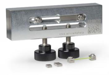
Alignment tool for sample preparation for measurements in tension mode
