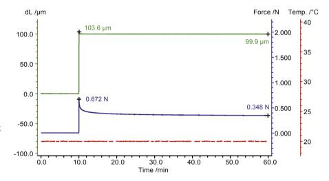
Relaxation measurement on an LDPE film, fused silica sample holder. Measured at room temperature under a nitrogen atmosphere; sample length 10 mm; sample width 5 mm.
