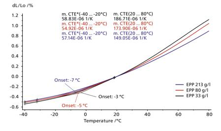
Expansion measurements on three different EPP foams with different densities. Sample length 20 mm, heating rate: 5 K/min from -40°C to 80°C under N<sub>2</sub> atmosphere, expansion sample holder made of fused silica and 50 mN sample load.
