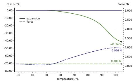
Measurement on a heat-shrink tubing under constant force (green curves) and under constant displacement (blue curves). Heating from RT to  $120^{\circ}$ C, atmosphere N<sub>2</sub>, sample length 25 mm (blue) and 10 mm (green).
