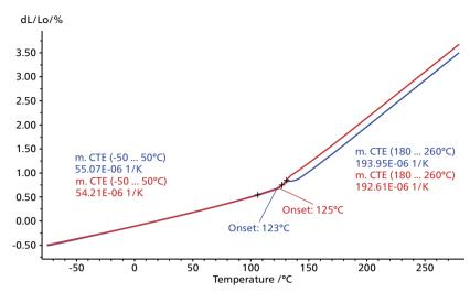
CTE measurement on an epoxy resin with a sample length of 6 mm in expansion mode (fused silica sample holder); 1<sup>st</sup> and 2<sup>nd</sup> heating runs at a rate of 2 K/min
