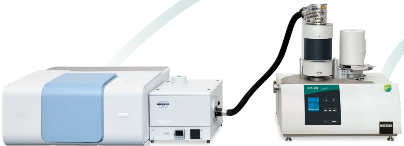
Bruker INVENIO with external gas cell
