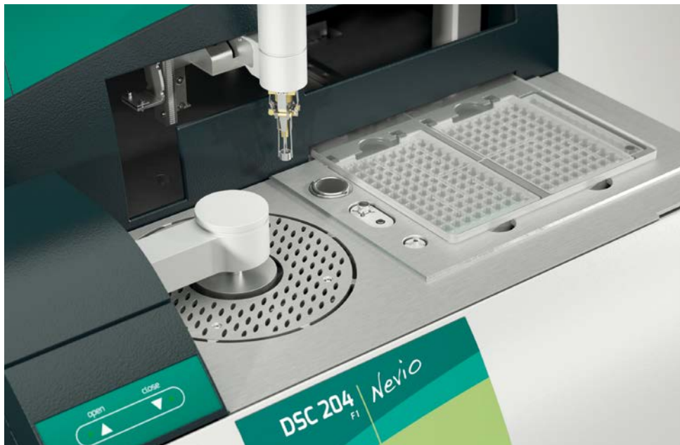
DSC 204 F1 Nevio with automatic sample changer (ASC)
