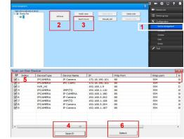
**★ Add device manually:** Configuration→Device Management →Add Manually
