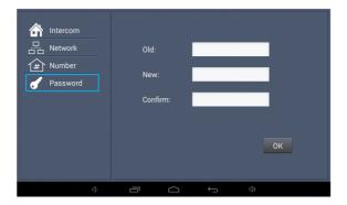
Click the input box after the old password, enter the original password through the numeric keypad that pops up, enter the new six-digit password in the same way and then re-enter the password in the box next to the item "Confirm". Clicking "OK", the system will emit a beep.
