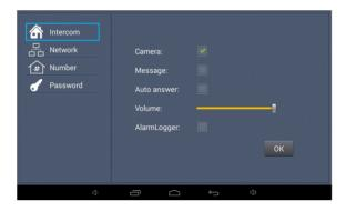
If you want to enable the functions of camera, automatic message, automatic answering and alarm logger, check the boxes, swipe left and right to adjust the intercom volume, and then click "OK" icon.
