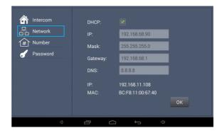
DHCP: When enabled, the router automatically allocates the IP address.
